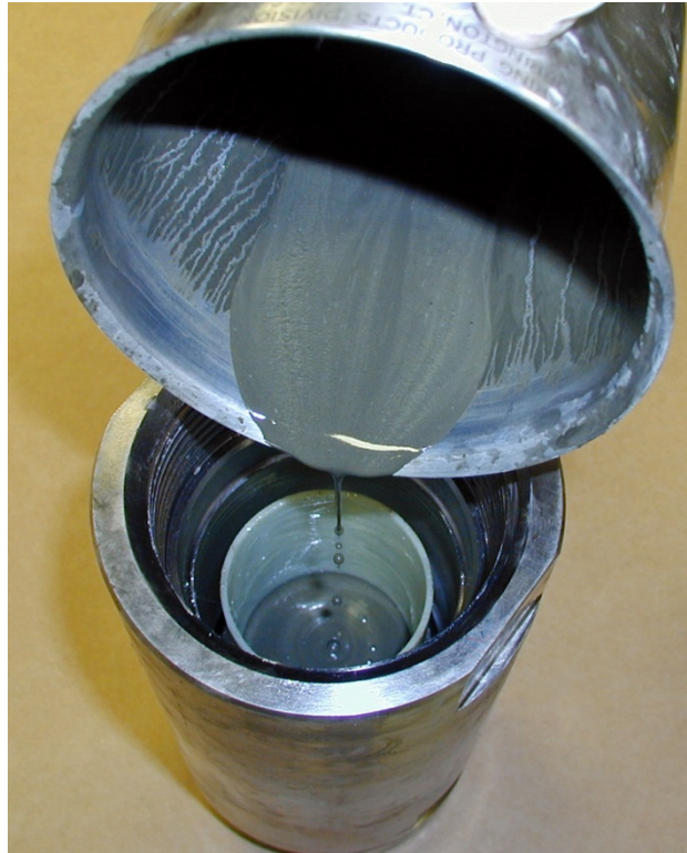
Figure 5-15 Pouring cement slurry into sample sleeve
