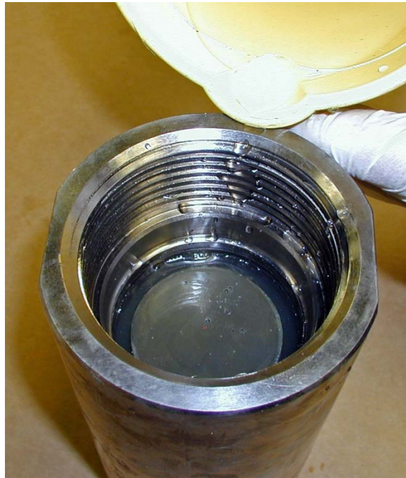
Figure 5-18 Water just covers the cement slurry
