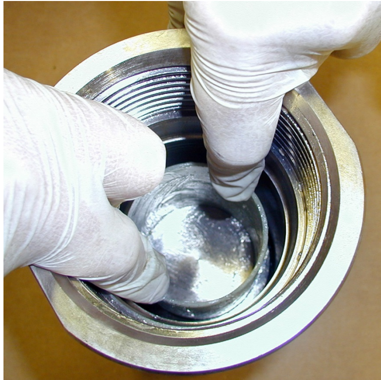
Figure 5-14 Seating sample sleeve into bottom lid groove
