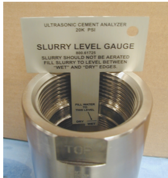
Figure 5-19 Slurry level gauge
