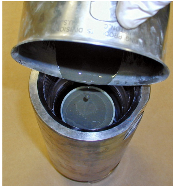
Figure 5-16 Fill the sample sleeve to the top
