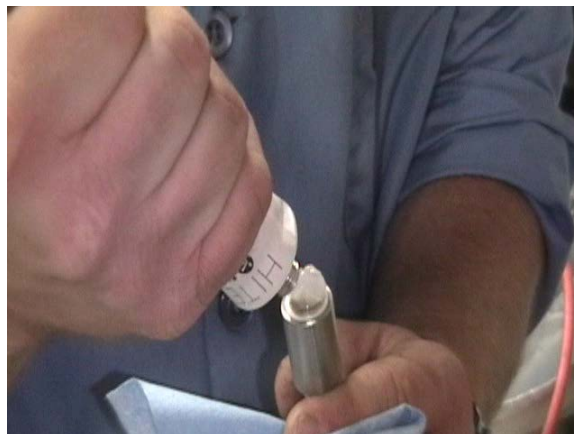
Figure 5-23 Coupling gel on transducer
