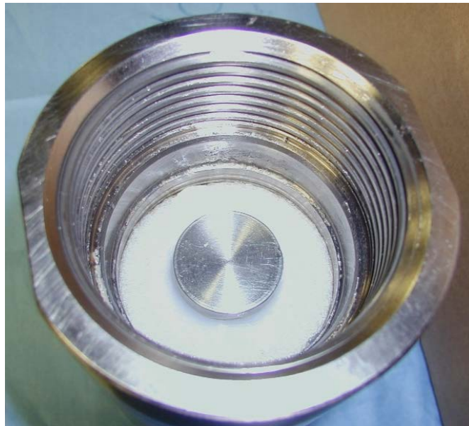
Figure 5-5 Calibration rod and foam centering ring in chamber
