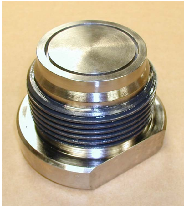
Figure 5-13 Groove in bottom test chamber lid for sample sleeve
