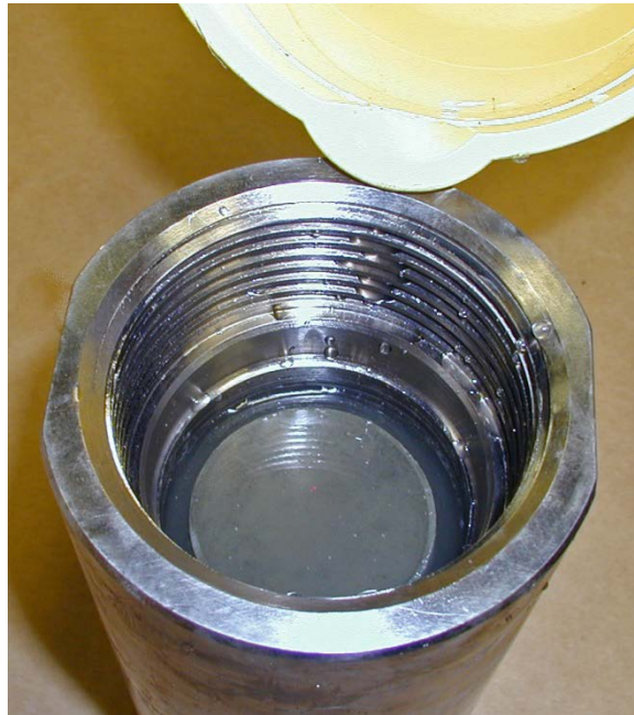
Figure 5-17 Pouring water around sample sleeve
