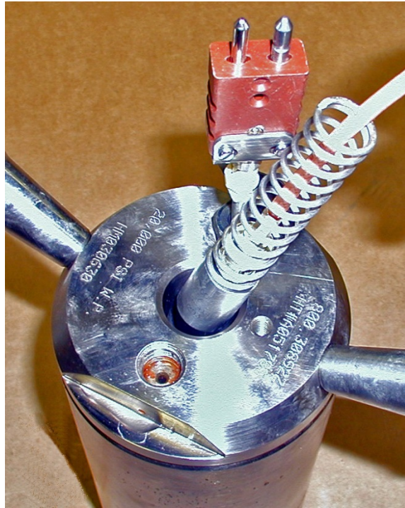
Figure 5-24 Inserting the transducer into the top lid
