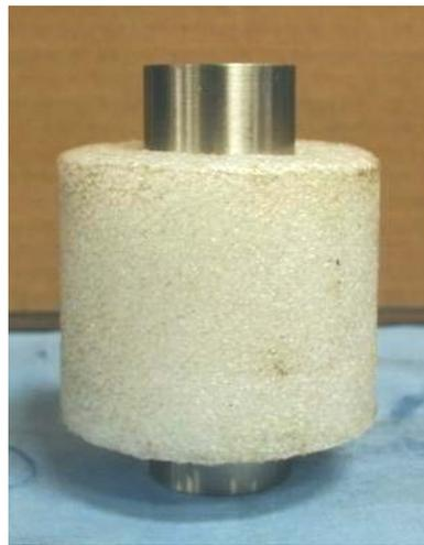
**Calibration rod and foam centering ring**
