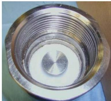
**Calibration rod and foam centering ring in the chamber**
