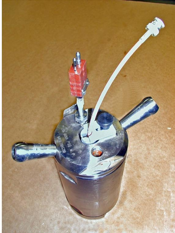
**Assembled test chamber with thermocouple and transducer**
