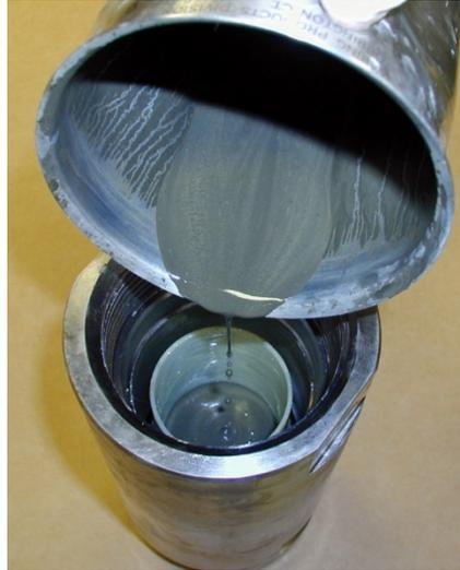
**Pouring cement slurry into sample sleeve**
