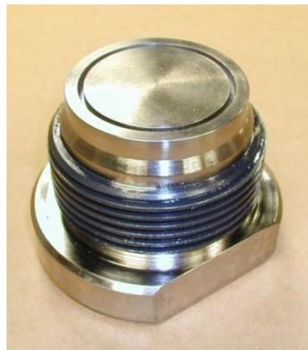
Groove in bottom test chamber lid for sample sleeve
