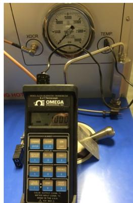
**Temperature calibrator connected for temperature calibration**
