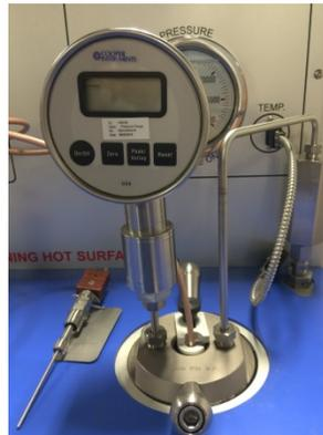
**Pressure gauge connected for pressure calibration**
