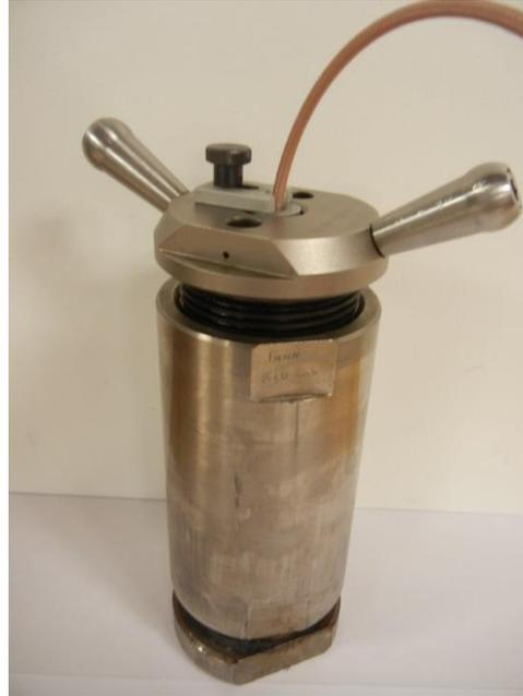
**Assembled test chamber with transducer**
