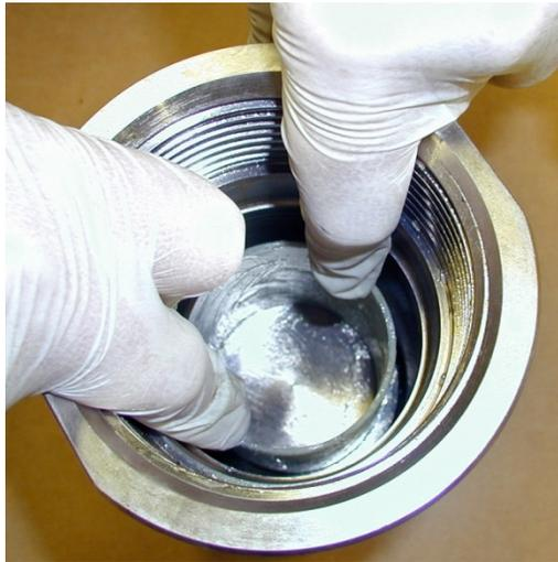
**Seating sample sleeve into bottom lid groove**
