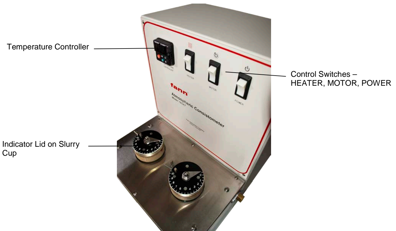
Figure 3-1 Model 165AT Atmospheric Consistometer
