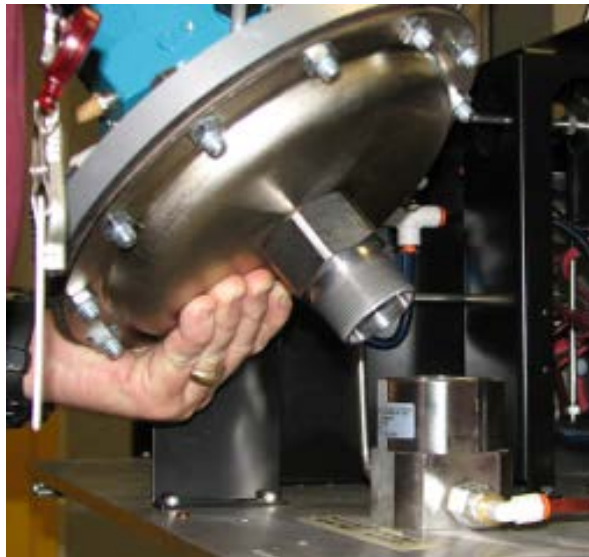
Figure 8-4 Removing Air Actuator Assembly
