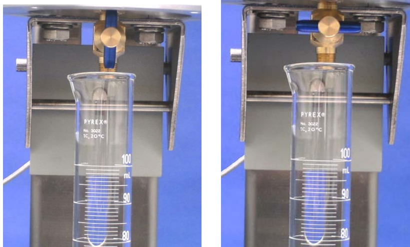
Figure 5-27 Bottom reservoir outlet valve (closed on left, open on right)
