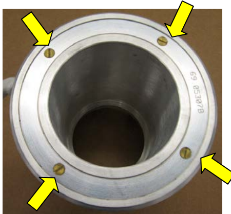
Figure 7-2 Heating element cover screws
