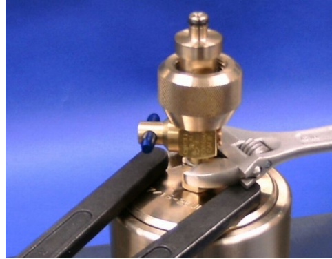
Figure 5-14 How to tighten top valve with adjustable wrench
