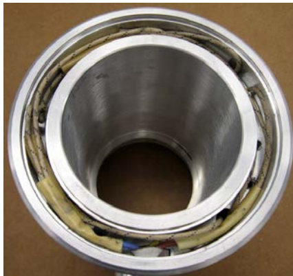
Figure 7-3 Heating elements and wiring exposed
