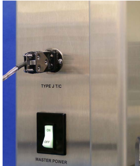
Figure 5-16 Heating Jacket Thermocouple plugs on left side of the instrument
