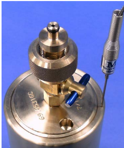
Figure 5-17 Cell Thermocouple partially inserted in reservoir
