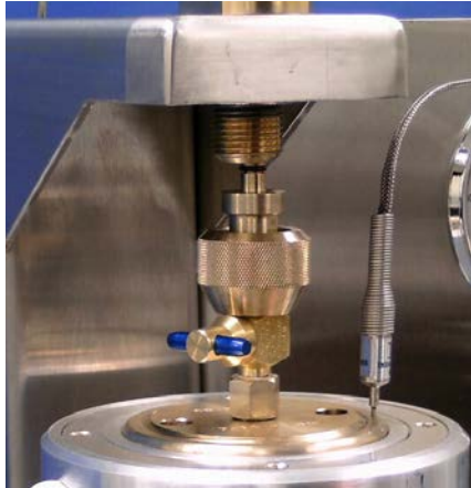
Figure 7-6 Correct height of heating jacket
