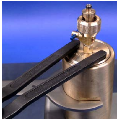
Figure 5-20 Tighten top cap with wrenches
