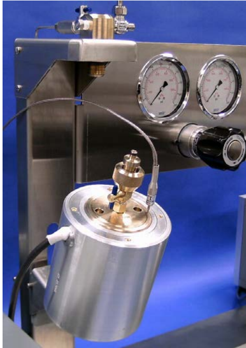
Figure 5-19 Reservoir in heating jacket for pre-heating
