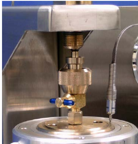
Figure 7-7 Correct height of heating jacket
