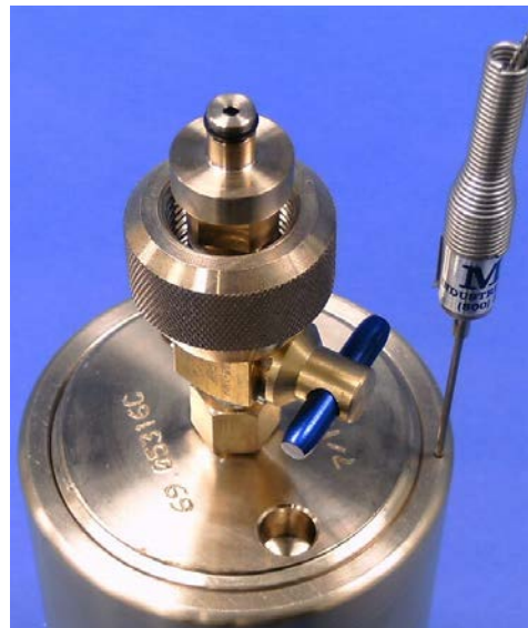
Figure 5-18 Thermocouple partially inserted in reservoir
