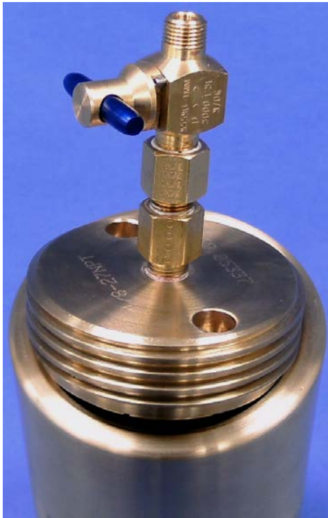
Figure 5-9 Install the bottom (grooved) reservoir cap
