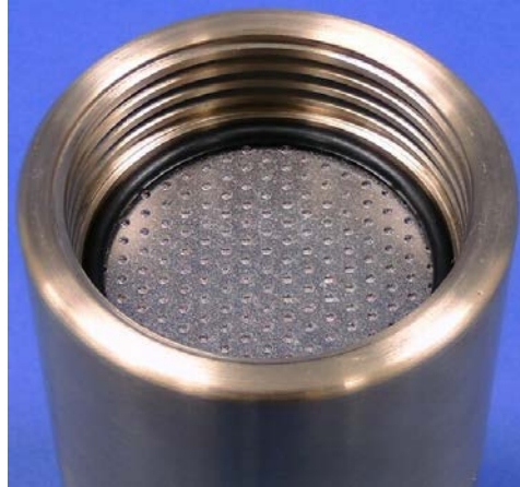
Figure 5-7 Screen and O-ring in reservoir bottom
