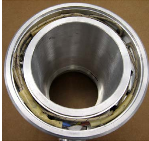
Figure 7-4 Heating elements and wiring exposed
