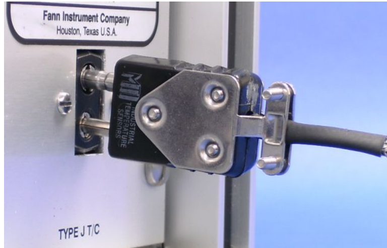
Figure 5-17 Thermocouple plugs in at the rear of the temperature controller
