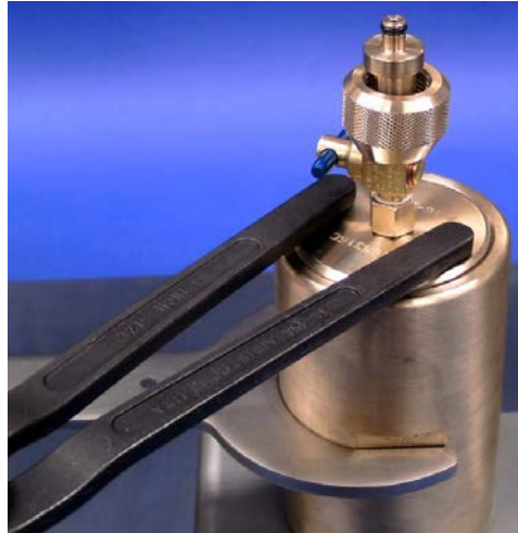
Figure 5-22 Tighten top cap with wrenches
