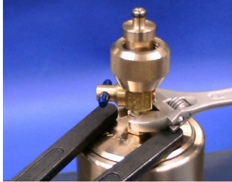
Figure 5-15 Tighten top valve with adjustable wrench
