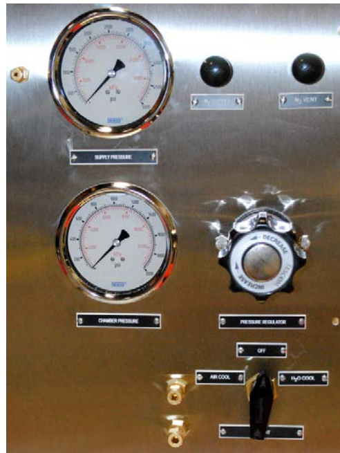
Figure 3-7 Pressure and Coolant Controls
