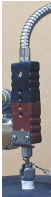
Figure 5-20 Connect thermocouple cable
