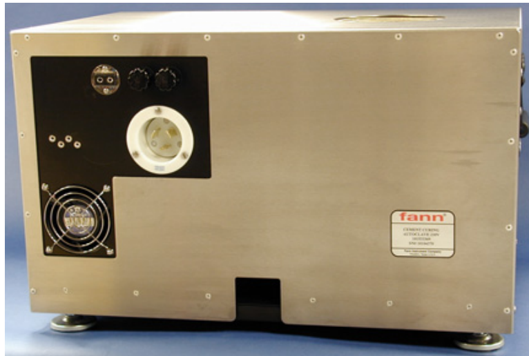
Figure 1-2 Cement Curing Autoclave, back view
