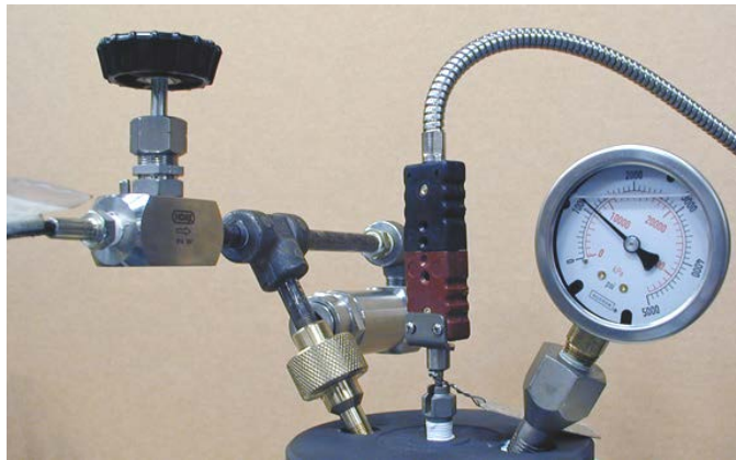
Figure 3-2 Pressure Manifold, Thermocouple, Pressure Gauge
