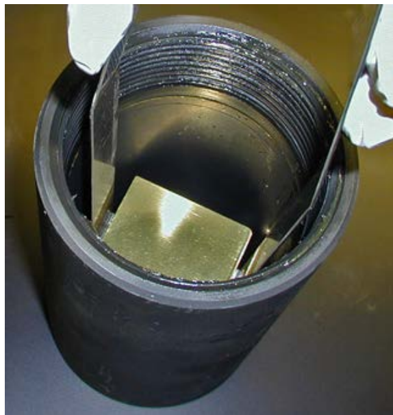
Figure 5-12 Lower mold into chamber – 2
