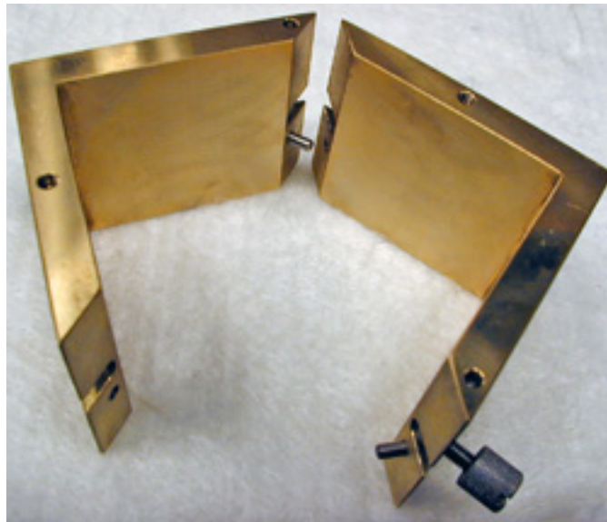
Figure 5-1 Pins align the mold halves
