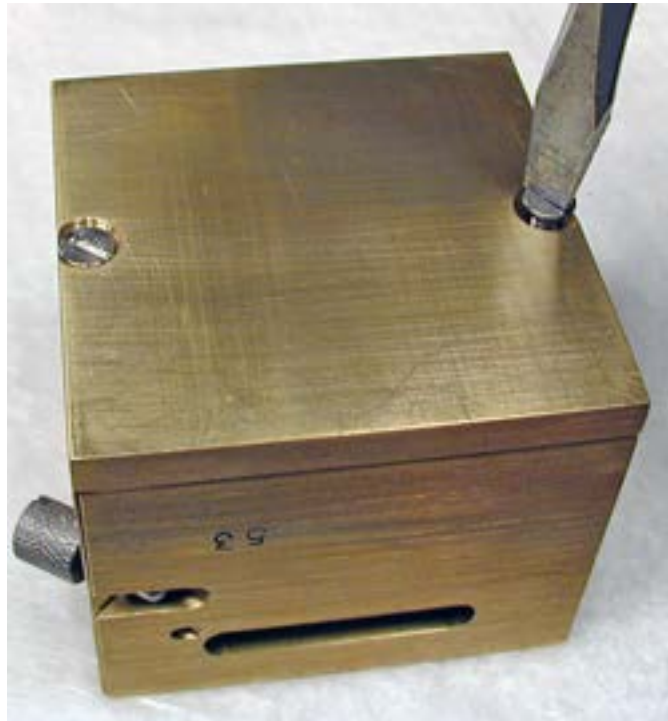
Figure 3-5 Cement Mold Base
