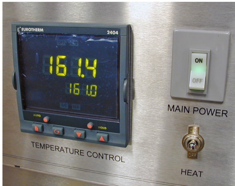
Figure 3-6 Temperature Controller, Main Power, Heat switch
