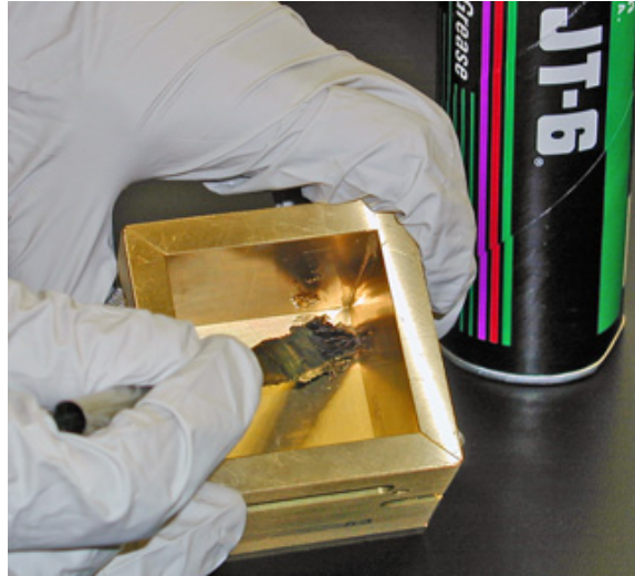
Figure 5-5 Grease mold interior
