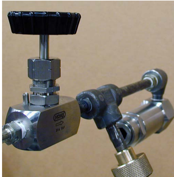
Figure 5-19 Attach valve and manifold
