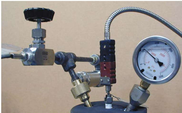
Figure 5-21 Set initial chamber pressure
