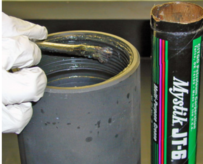
Figure 5-13 Grease chamber threads
