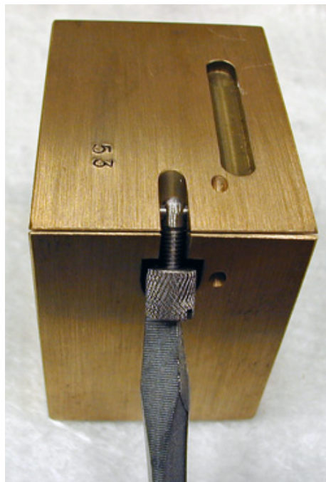
Figure 3-4 Cement Mold Clamp
