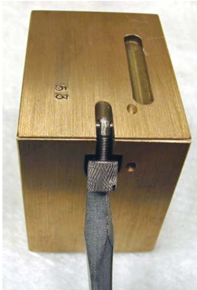
Figure 5-2 Clamps hold mold halves together
