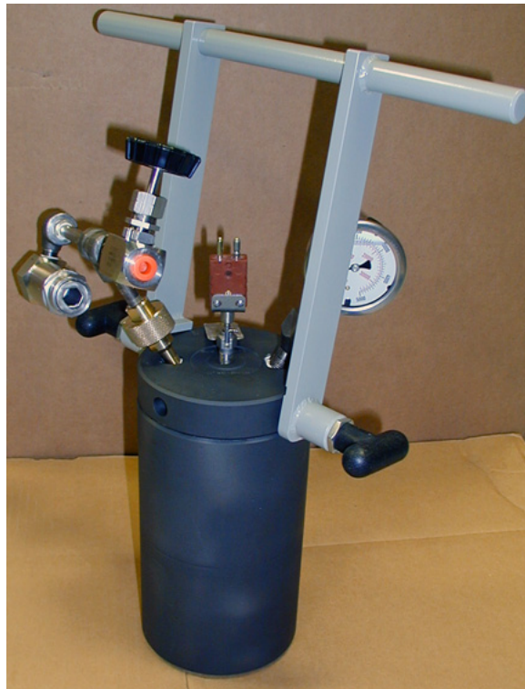
Figure 5-17 Handle and manifold on chamber
