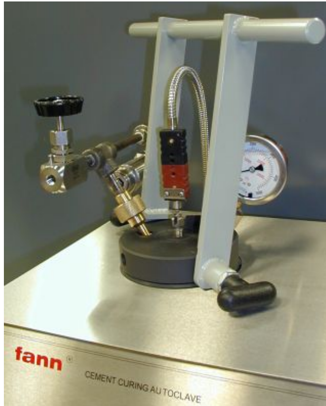
Figure 5-18 Place chamber into autoclave, remove handle
