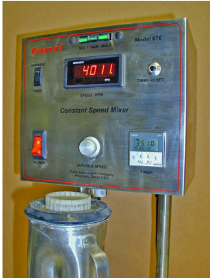
Figure 5-6 Mixing Cement Slurry
