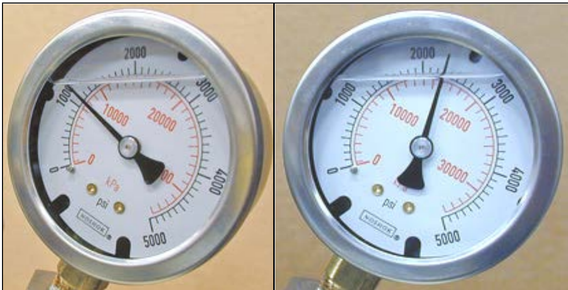
Figure 3-9 Initial pressure (left), increased pressure from temperature rise (right)
