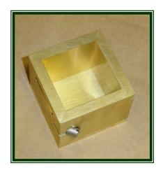
The Single Cube Mold is designed and manufactured to form 2" (50.8 mm) single cube samples for compressive strength testing. Mechanical screw clamps are used to connect the two halves of the mold so they can be drawn tightly together. The clamping screws are held in place by a pin, which allows rotation of the screws for ease of assembly/disassembly, prevents loss. Carefully machined, smooth surfaces facilitate cleaning of the mold.
