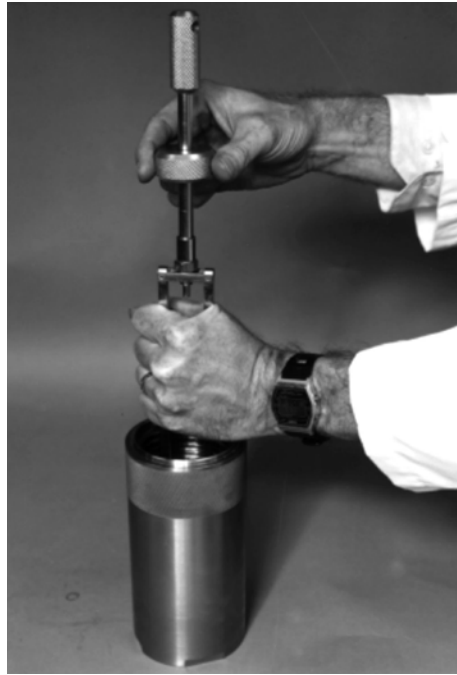
Figure 5-51 Removing the bushing inner race or the pivot bushing
