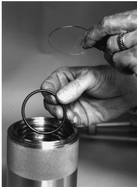
Figure 5-39 Installing the cell seal O-ring and its backup ring
