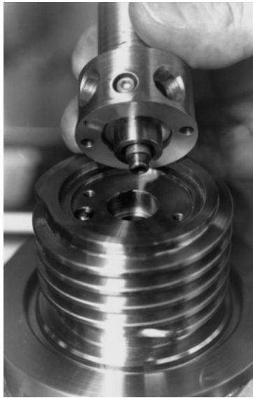
Figure 5-47 Location and orientation of the ball under the torsion spring module
