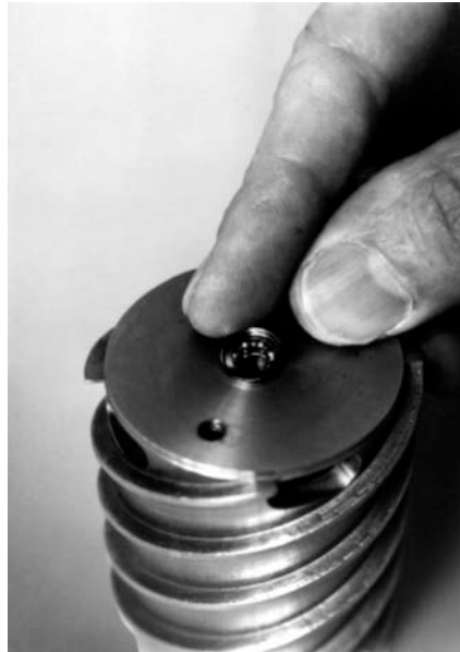
Figure 5-50 Placing the bushing outer race in place for pressing
