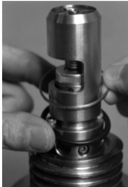
Figure 5-42 Installing the cap seal O-ring and backup ring
