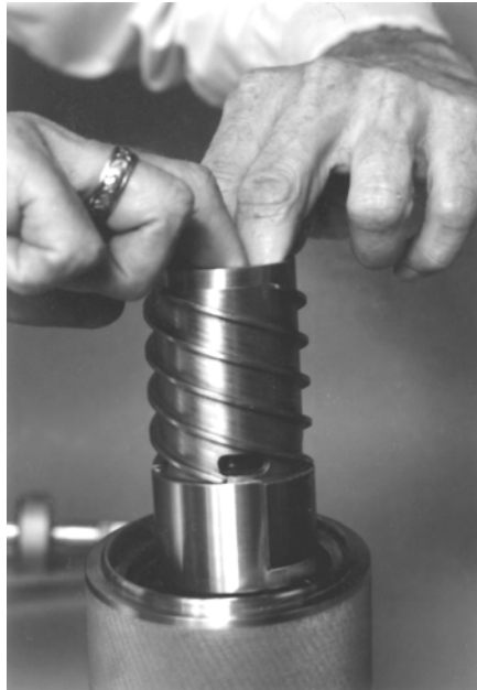
Figure 5-32 Installing rotor in cell
