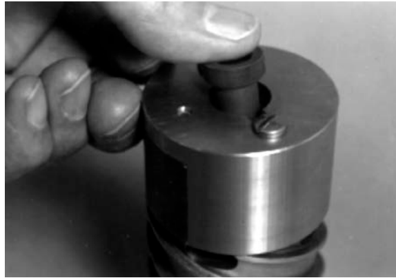
Figure 5-55 Pushing the rotor bushing into position
