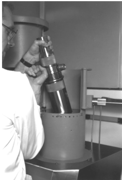
Figure 5-35 Placing the test cell into the hot well
