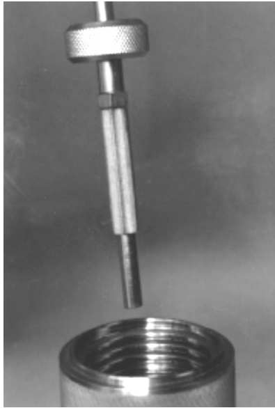
Figure 5-53 Pushing the inner race onto the pivot
