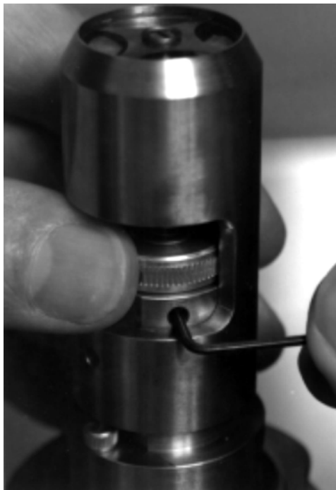
Figure 5-59 Adjusting the zeroing sleeve
