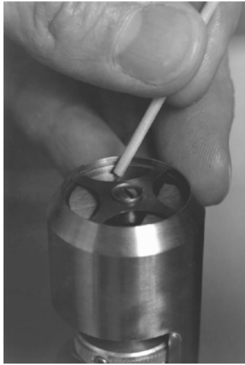
Figure 5-34 Checking for free rotation of the torsion assembly
