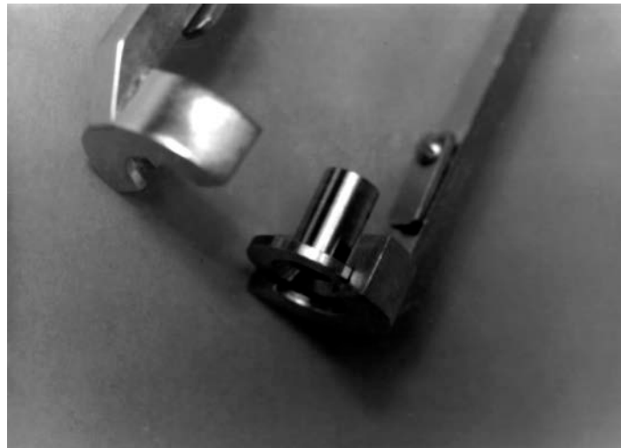
Figure 5-57 The Pivot Bushing in the groove of the Puller
