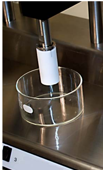
Figure 5-11 Evaporation Dish under the Measuring Head
