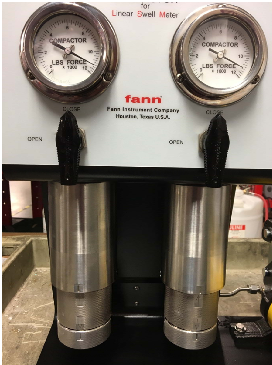
Figure 5-4 Panel Valve And Pressure Gauge on Compactor Cell
