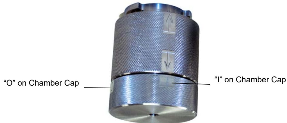
Figure 5-1 Compactor Cell with Core Sample
