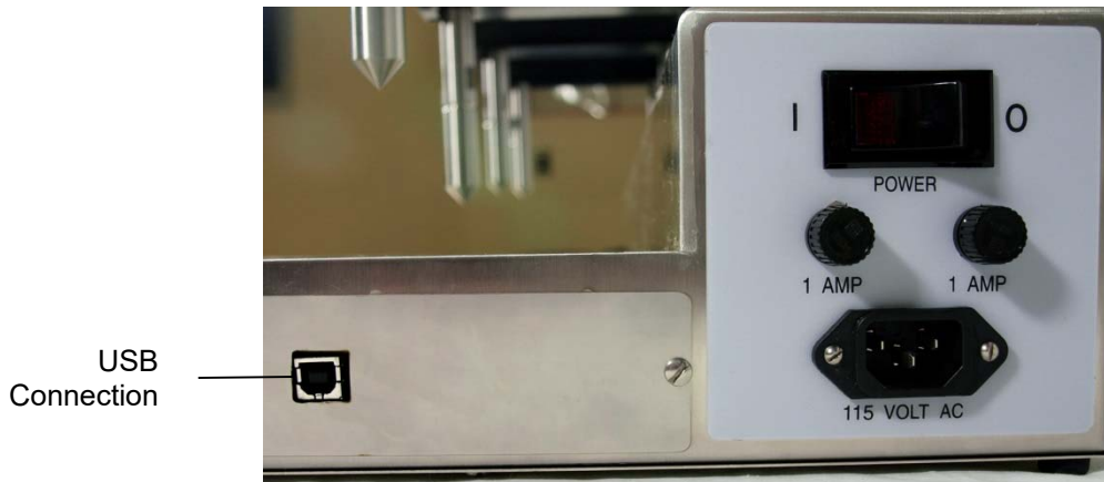
Figure 4-1 Computer Connection on LSM
