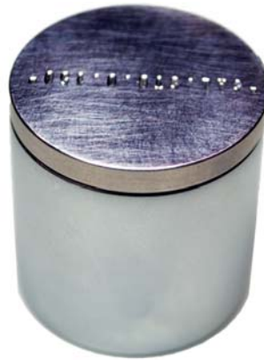
Figure 5-8 Calibration Disk on Spacer Block
