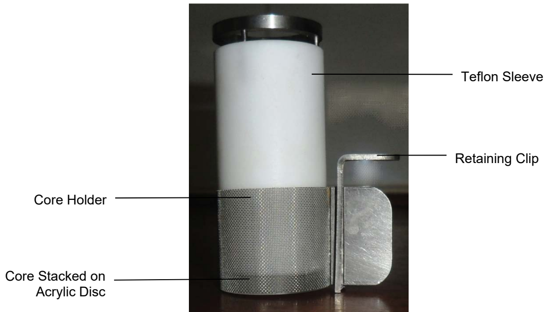
Figure 5-10 Spacer and Core Plug Stacked in Core Holder
