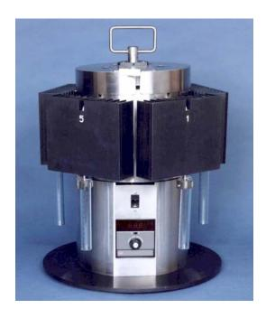
The *Multi-Retort* is a 5-cell; 50ml <u>oil and water retort</u> which allows more accurate, faster, consistent, and convenient gathering of oil on cuttings data as well as oil, water, and solids analysis of drilling fluids.
