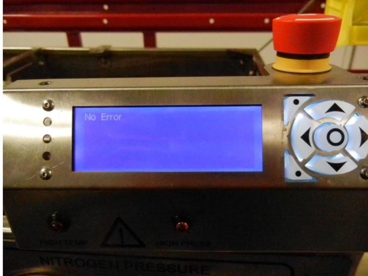
b. If there is an error it looks like below. Press the center button to clear the error. The red LED will be on if there is an error message available. In the picture below this error occurred because the user tried to fill the system though the system did not have the auto filtrate installed setting selected.
