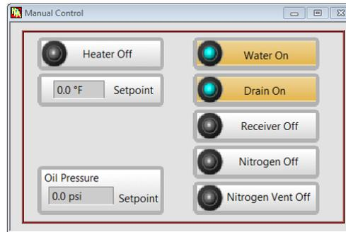
4. The pump should turn on, and water will begin to flow through the system. Bubbles will flow through the drain sight tube as water exits to the drain. Click on the buttons again to close the valves.
