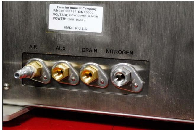
**Figure 4-2 Connection Ports on the Back Panel**
