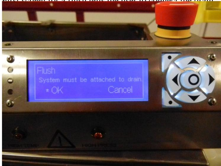
2. Since flush can run automatically the flush screens consist of messages describing the current step
