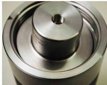
Figure 4-4 Cap Retainer installed
