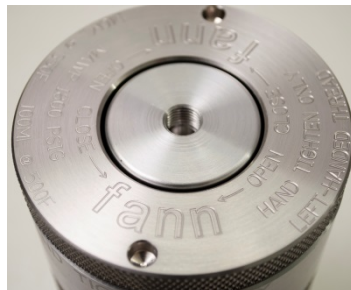
Figure 4-5 Cell Cap installed
