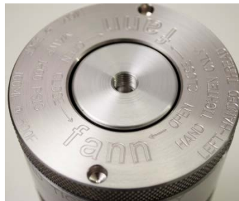
Figure 5-4 Cell Cap installed
