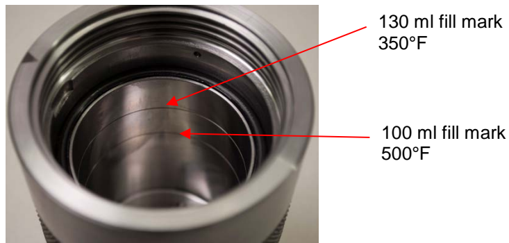
Figure 5-1 Cell showing fill marks inside
