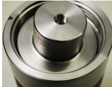
Figure 5-3 Cap Retainer installed
