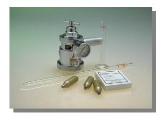
The Half Area Filter Press is a compact version of the standard Filter Press and employs 1/2 size filtration area. Time and pressure requirements are the same as for the API filter press. Readings are converted to standard measure by multiplying by two as specified in the *American Petroleum Institute*, "API Recommended Practice 13B-1 and 13B-2".
