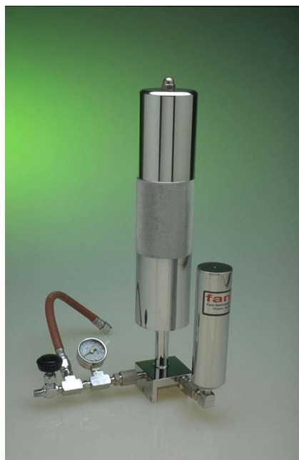
Hydraulic Dead Weight Assembly
