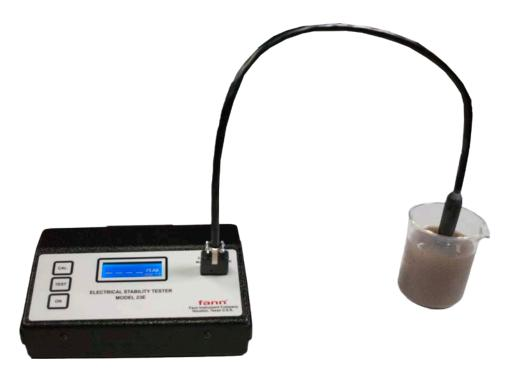
Figure 5-2 EST Probe immersed in sample
