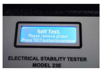
Figure 5-1 Self Test Mode
