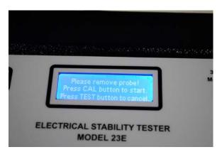
Figure 6-2 Self Calibration Mode
