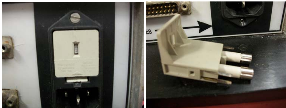
Figure 7-3 Fuse Drawer in place (left) and removed (right)
