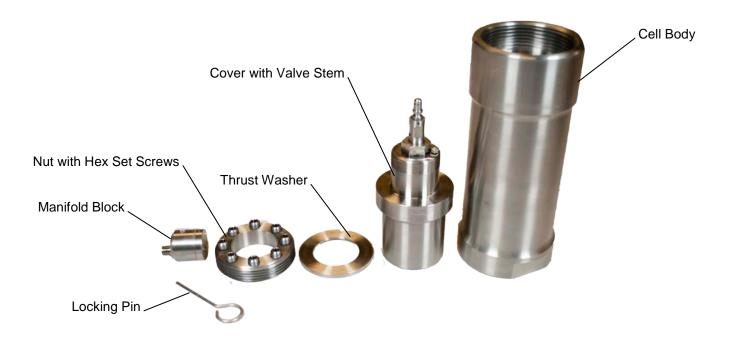
Figure 3-1 600°F High Temperature Aging Cell
