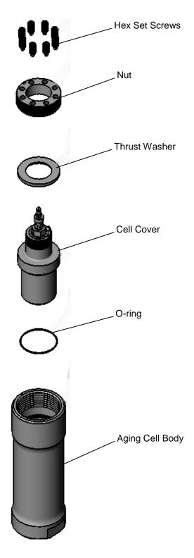
Figure 4-1 Unpressurized Aging Cell Assembly
