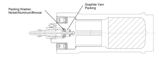
Figure 7-1 Cell Assembly Drawing
