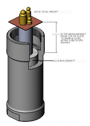
Figure 6-1 Shear Tube on Sample
