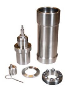
Figure 9-1 600°F Aging Cell Assembly
