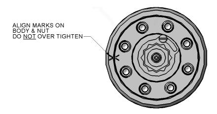
7. Use the 7/32-in. Allen wrench to tighten the center set screws into the nut.
