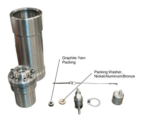
Figure 7-2 Disassembled Cell
